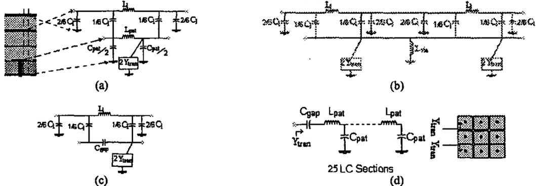
**Fig. 2** – Equivalent circuit for a transmission line with an EBG ground plane: (a) Patch section, (b) via sections, (c) gap section, and (d) the equivalent circuit representing the transverse loading.
