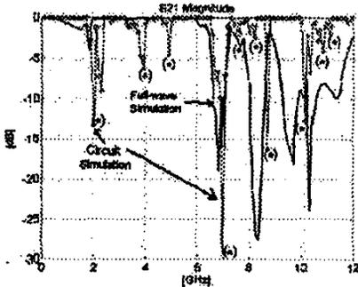
Fig. 4 –  $S_{21}$  simulation of circuit model.
