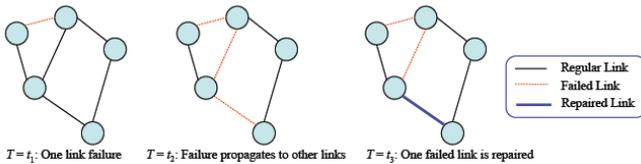
Fig. 1. Example of cascading failures and repairing.
